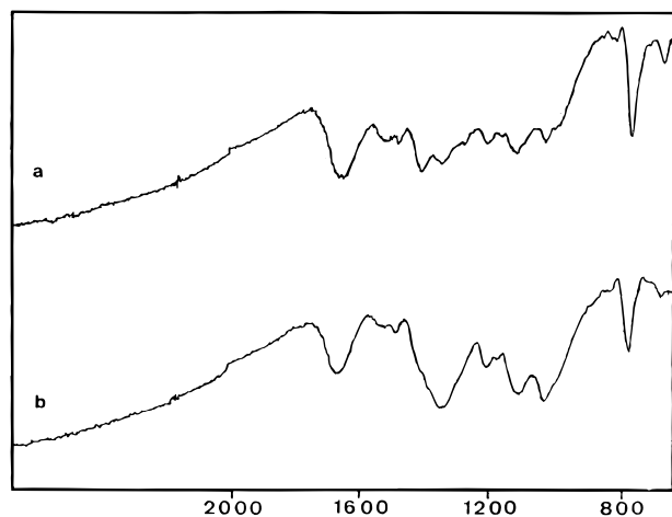
Figure 2. Infrared spectra in KBr pellets of (a) as-synthesized polymer and (b) I 2 -doped polymer from thiophene ( 3 ).
